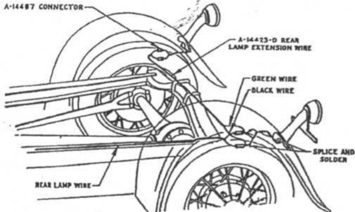
CUT OFF A-14483 TERMINALS FROM EXTENSION WIRE THEN SPlice AND SOLDER THE GREEN WIRE IN THE EXTENSION TO THE GREEN WIRE EXTENDING FROM THE TAIL LAMP, THEN CONNECT THE BLACK WIRES IN THE SAME MANNER AND TAPE BOTH CONNECTIONS
